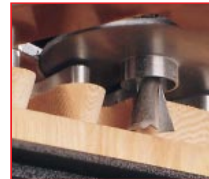
The dovetail profile is formed using the TCT cutter supplied with the jig. The guide bush fitted to the router, follows the fingers of the template.
