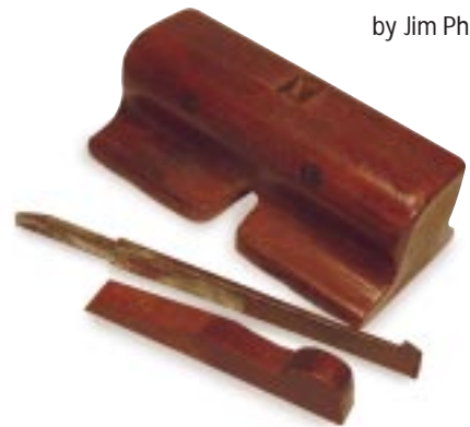
A 'tooth', forerunner of today's router cutter.
