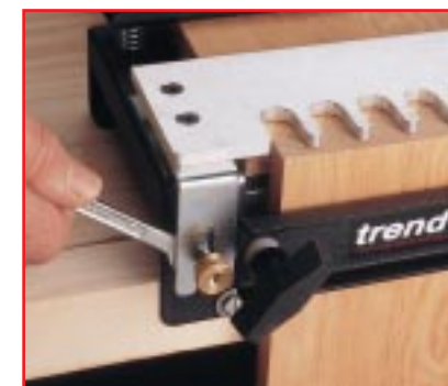
The position of the template is adjusted using the spanner supplied to set the depth of the dovetail joint.
