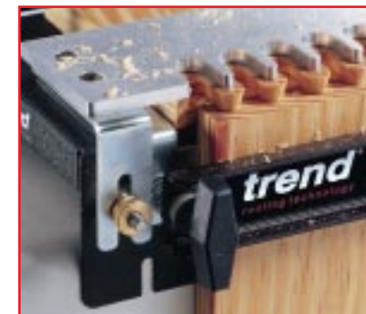
Once the router is set up correctly, it will cut both pins and tails in one pass.
