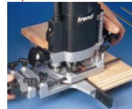
Edge moulding using the side fence as a guide.
