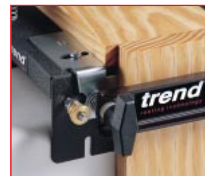
The timber is positioned tight up against the edge guide to fix the joint off-set. The side of this draw assembly is placed in the front clamp and the front of the drawer is placed in the top clamp.
