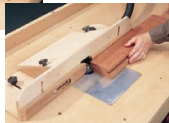
A simple fence can be made from plywood and fitted with adjustable faces.
