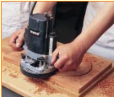
Forming the mirror frame with the Mini Ellipse Jig
